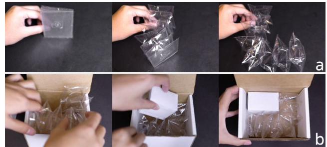
Figure 13: Customized Air Pillow: (a) A customized L-shape air pillow (b) It ideally fills the entirety of the empty space within the packaging.
