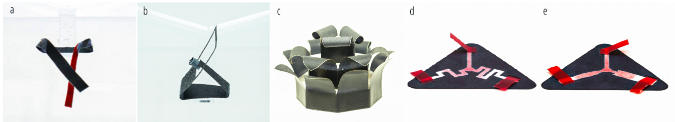
Figure 1: Application demonstrations. (a) Morphing strip - a strip that can sequentially fold with 45 degrees folding angles; (b) Self-locking structure - a structure with gray levels on different regions that can self lock and unlock itself; (c) Morphing flower - a flower with different gray levels petals that can boom in sequences; (d) Triggered length primitive; (e) Triggered width primitive.
