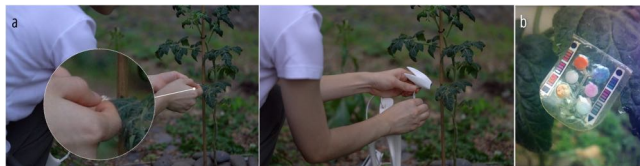
Figure 11: (a) The user is deploying the guttation chip and camera module at dusk, then waters the plant well. (b) Detection result captured by the camera on the next morning.
