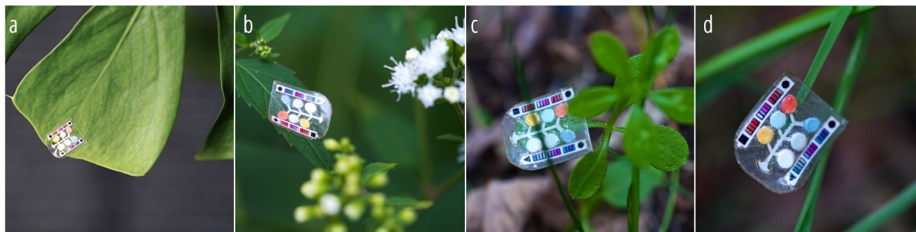
Figure 13: The guttation chip can be mounted to and be held on various plant leaves. From the large and thick Monstera deliciosa leaf (a), to thin and sharp grass leaf (d).
