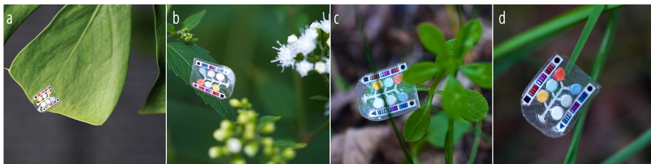
Figure 1: The guttation sensors mounted to various plant leaves. From the large and thick Monstera deliciosa leaf (a), to thin and sharp grass leaf (d).
